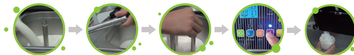
01 Pull the material 02 Close air tube 03 Insert air tube 04 Press AUTO 05 Making ice cream
