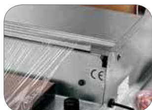
1. Particolare filo caldo (1) Heated cutting tread (1)
