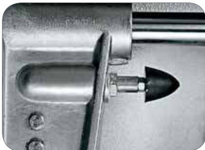
11. Paracolpo carrello Hopper's buffer
